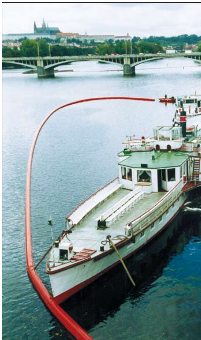
When applied on water, the bigger top chamber is filled with the air and the bottom chamber is filled with water
