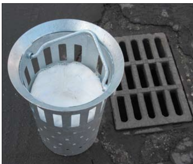
Compound fibers REO Fb have been used for the removal of hydraulic oil from the cooling stack pool of electric plant
