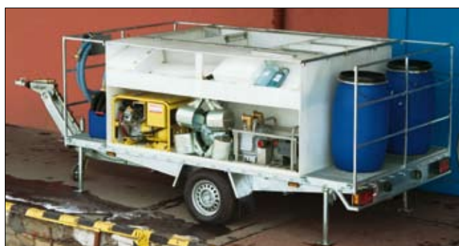
Mobile oil separator REO100 was used for a treatment of the oil phase from water surface inside the catch lagoons during the removal of the oil pipeline Družba breakdown in Čáslav on 9. 2. 2005.
