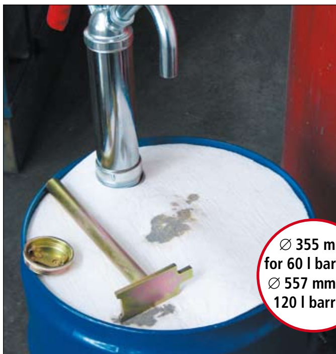
Pad absorbs pump drips during a pumping of liquids from standing barrel
